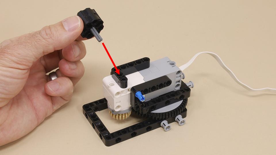
You can use this knob – to manually adjust the angle of the turntable.
