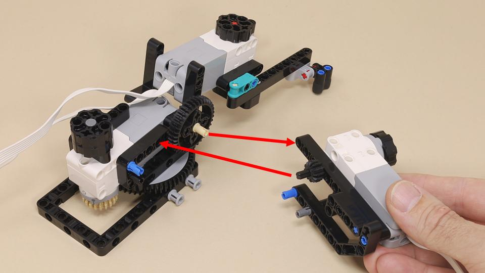
Hold the claw level while inserting the geared lift motor assembly.
