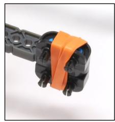
Wrap a rubber band three times around each claw end.
