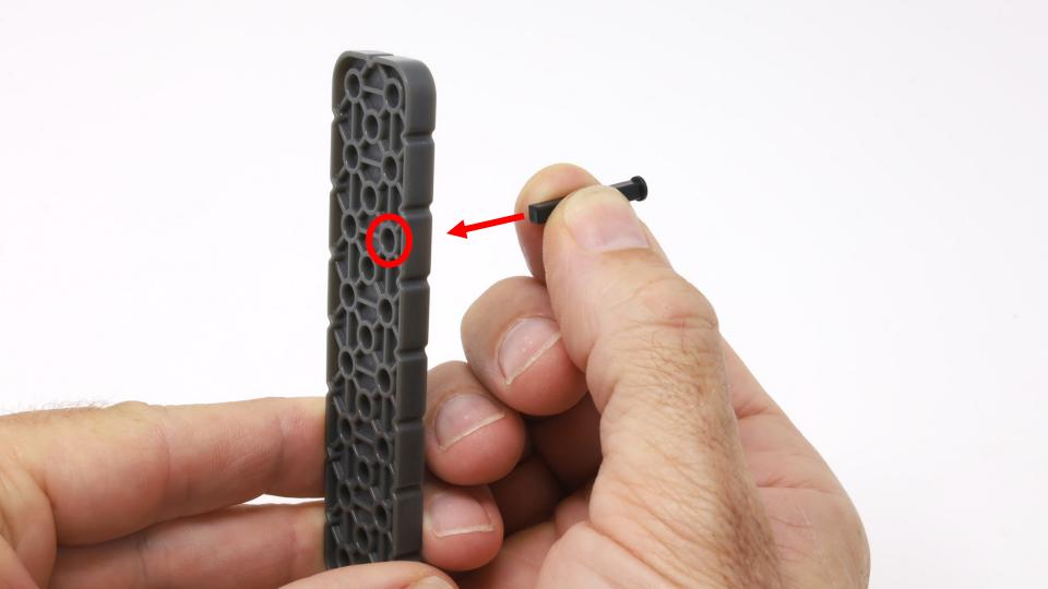
Hold this axle in with your finger while you guide the plate down over the motor axle.
