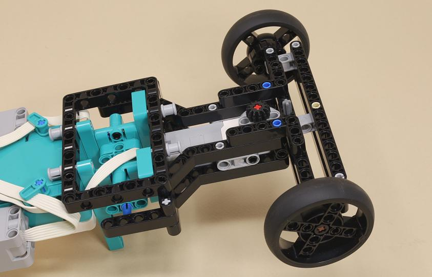
Because of the gears, it is not possible to get the wheels perfectly straight with the steering motor in its zero position. Keep the motor aligned to its zero position, then insert the beige gear with the wheels as close to straight as possible, with the slight error in the direction shown below.
