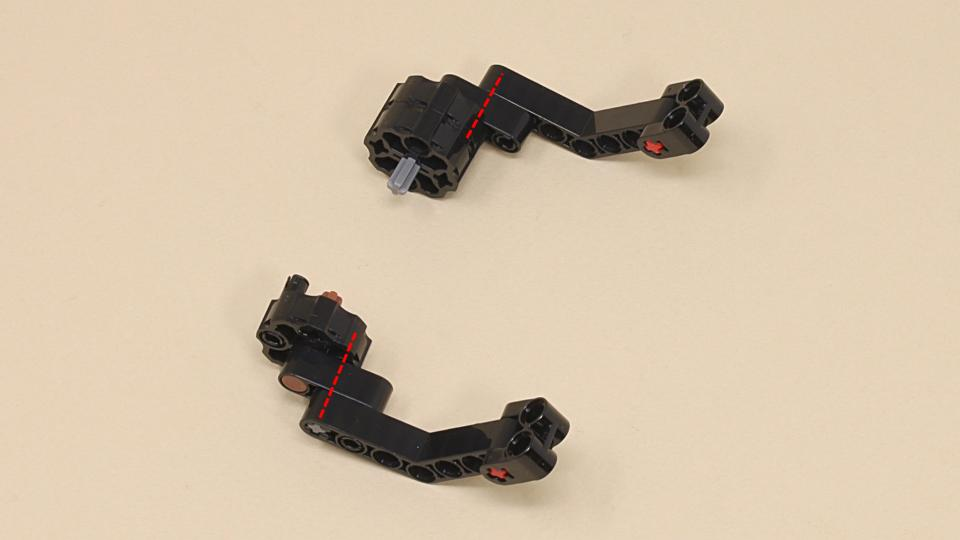
The back part of the arms should be vertical when the arm motor is in its zero position.
