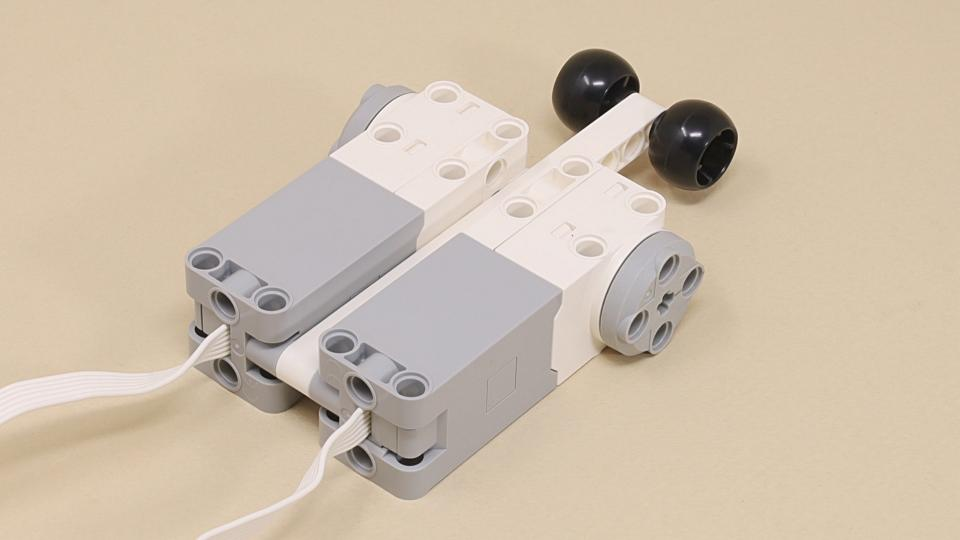
Make sure the distance sensor and arm motor wires stay out of the way.
