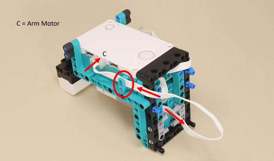
Fold and push the remainder of the arm motor wire under here.
