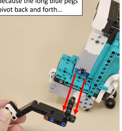
If you have trouble, you can push out the blue pegs, insert the short ends into the leg, and try it this way:
