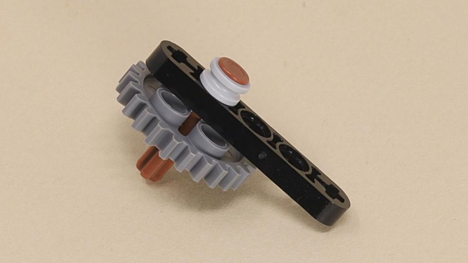
The compound gearing causes one turn of the motor to turn the output axle 9 times. To reduce friction with high gearing, make sure the parts are not pushed together too tightly. Slightly loose is better.
